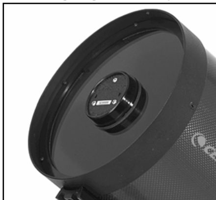
Figure 1-10 The three collimation screws are located on the front of the secondary mirror housing.
