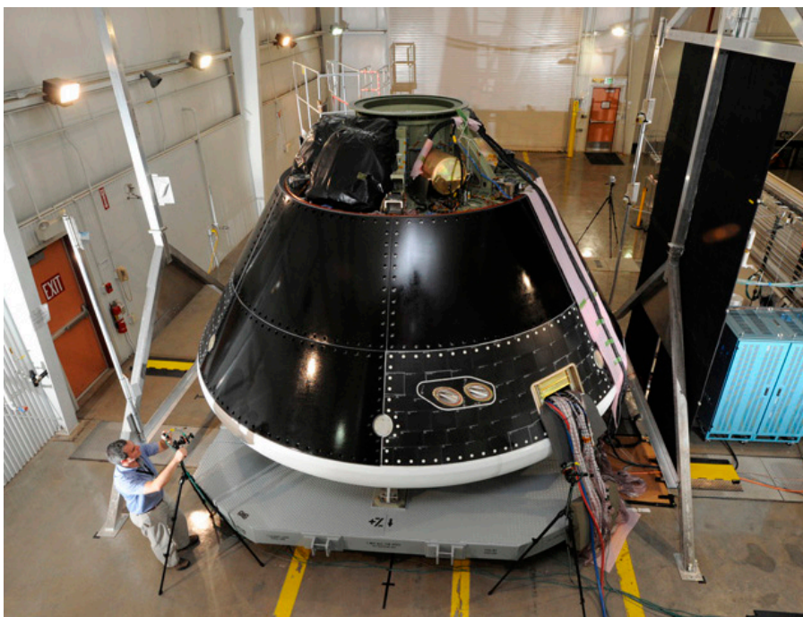
The Multi-Purpose Crew Vehicle being assembled and tested at Lockheed Martin's Vertical Testing Facility in Colorado. Photo credit: Lockheed Martin
